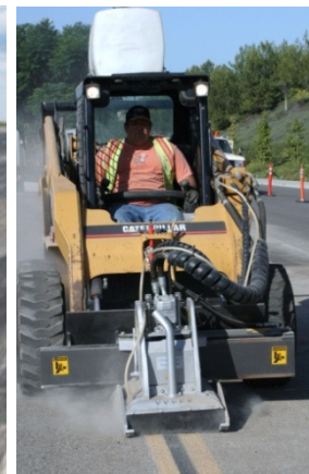
Skid-steer driven planer/grinder for up to 3,000 lf per hour
